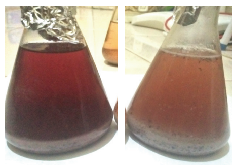
Figure 1. Color comparison of extraction process between ethanol (left) and aquadest (right).
